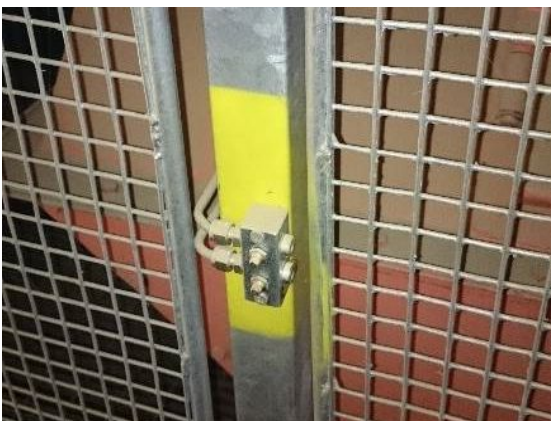
2 outlet grease anchor block
