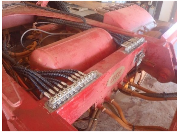
5 x 5 grease anchor blocks
